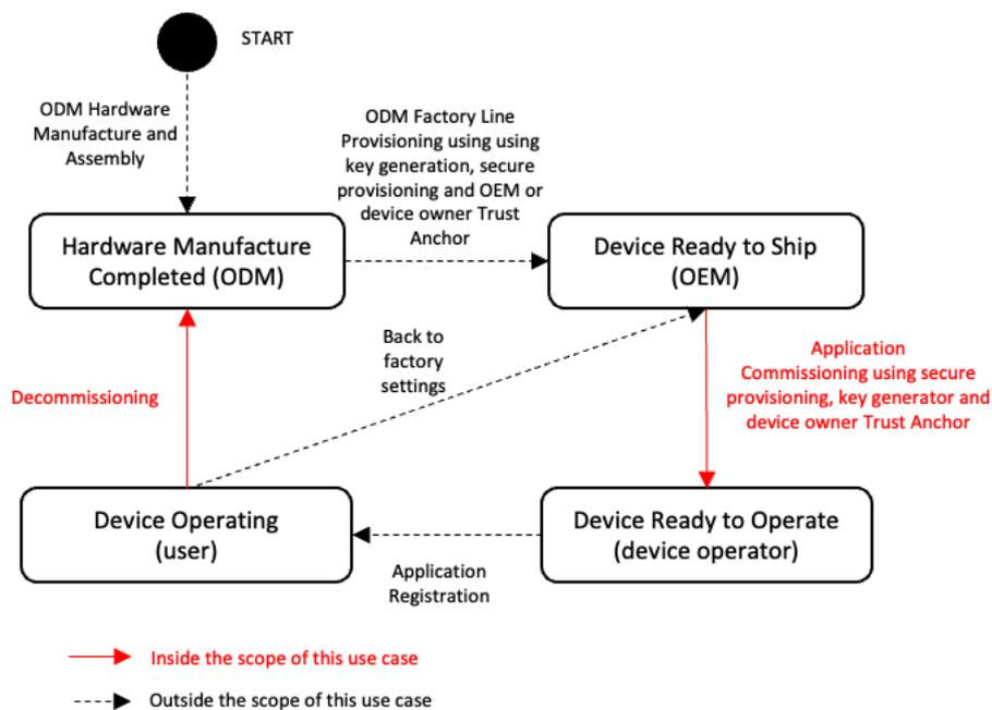
Figure 9: UC3 IoT Device Lifecycle Commissioning and Decommissioning Processes
