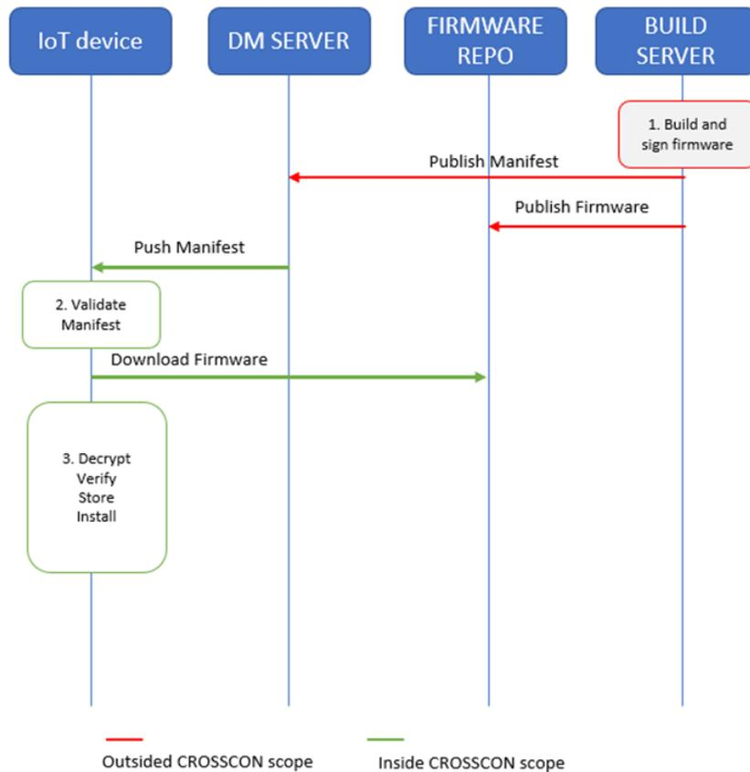
Figure 7: UC2 Typical IoT device firmware update process
