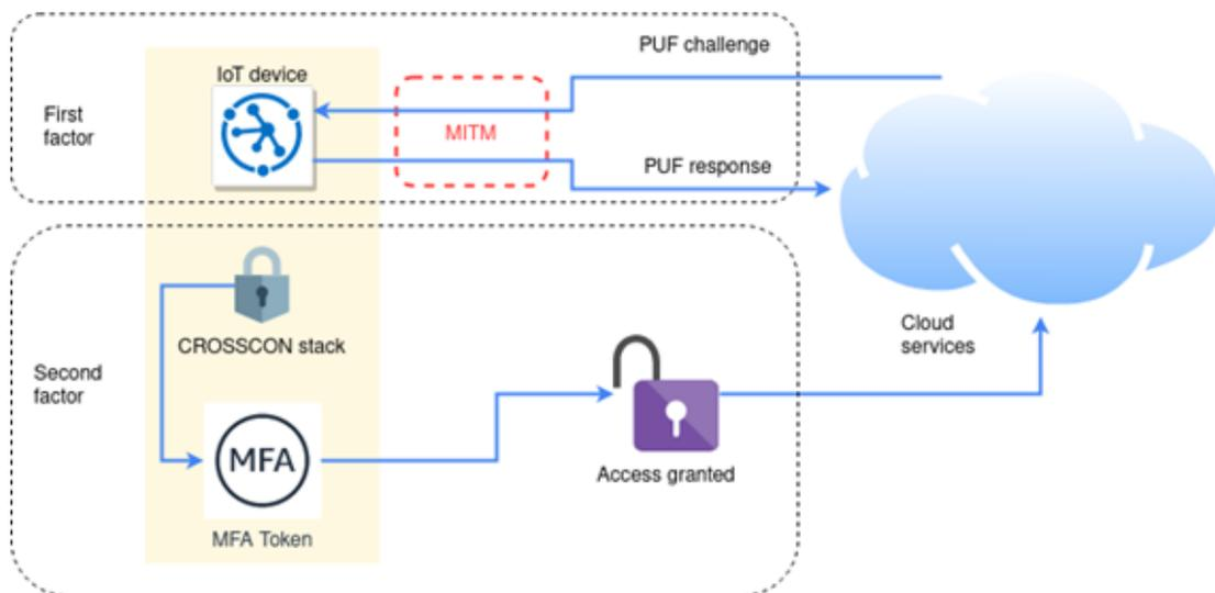
Figure 1: UC1 Device MFA High-level View
