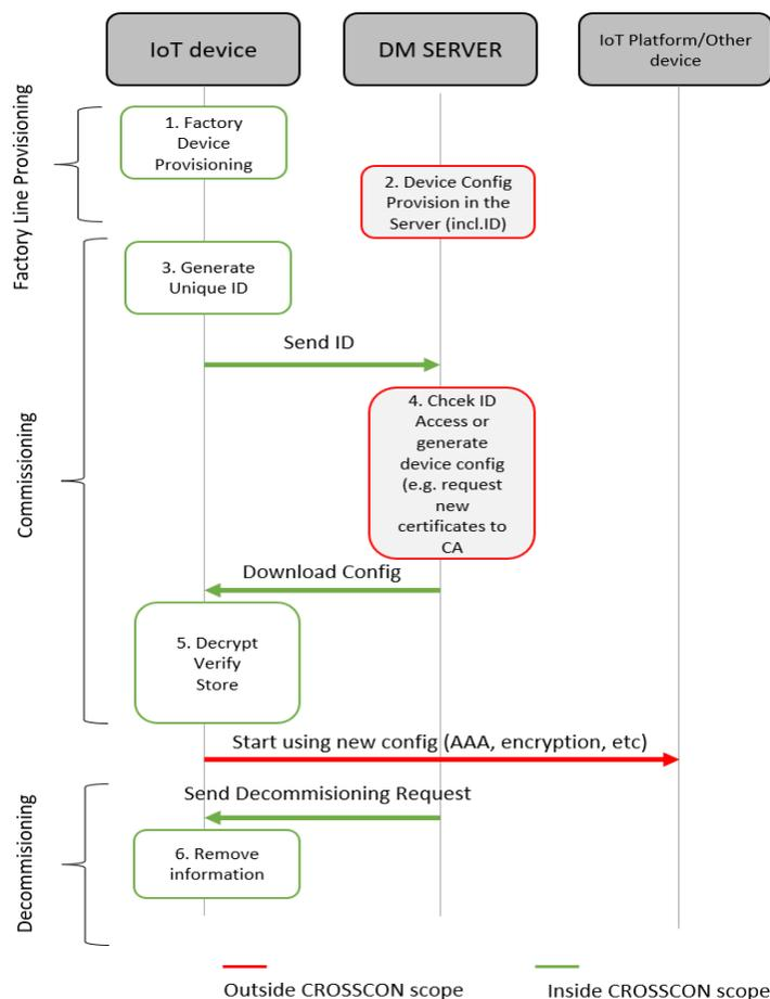
Figure 10: UC3 Commissioning and Decommissioning Processes Workflow
